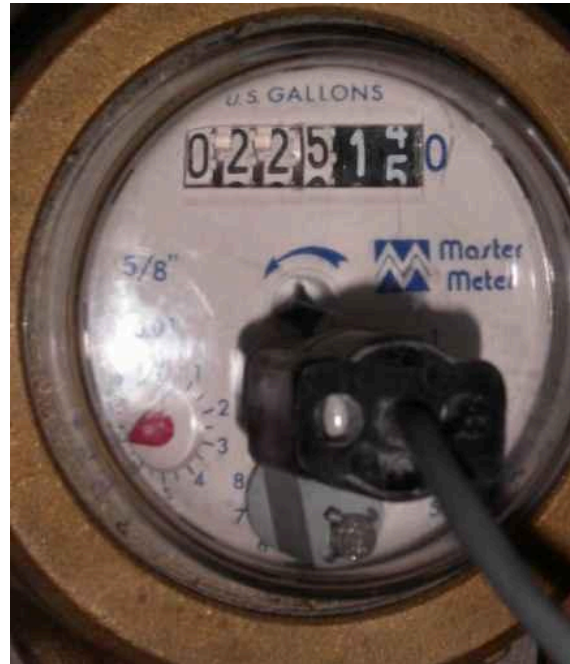
Figure 3 Meter with remote transmitter attached.
